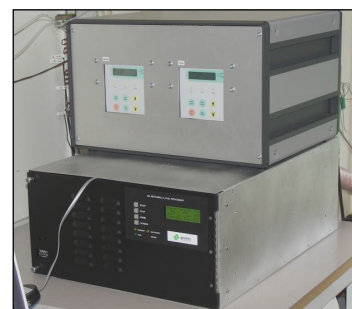
Photo: Tested methanol reformer with Cellkraft fuel mixer (top).
